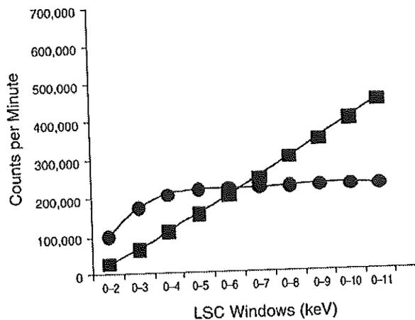
Figure A.3. Window energy optimization for liquid scintillation counter (LSC). <sup>54</sup>Mn produces Cerenkov radiation that overlaps with the LSC energy window for <sup>14</sup>C. Two replicates of <sup>54</sup>Mn (●) and <sup>14</sup>C-sucrose (■) were repeatedly counted at energies of 0–2 keV to 0–11 keV. Results are expressed in counts per minute.
