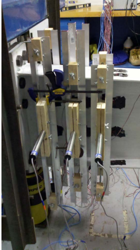
Figure C-1 LVDTs Near Failure Location
