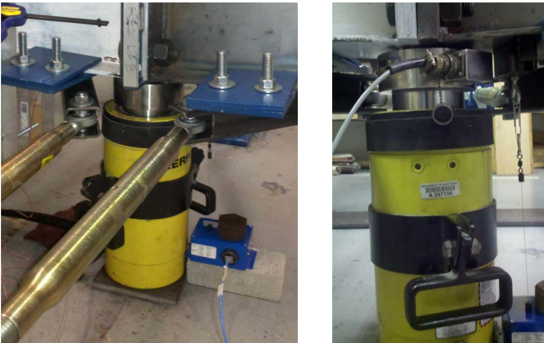
Figure 2-5 Hydraulic Ram and Load Cell
