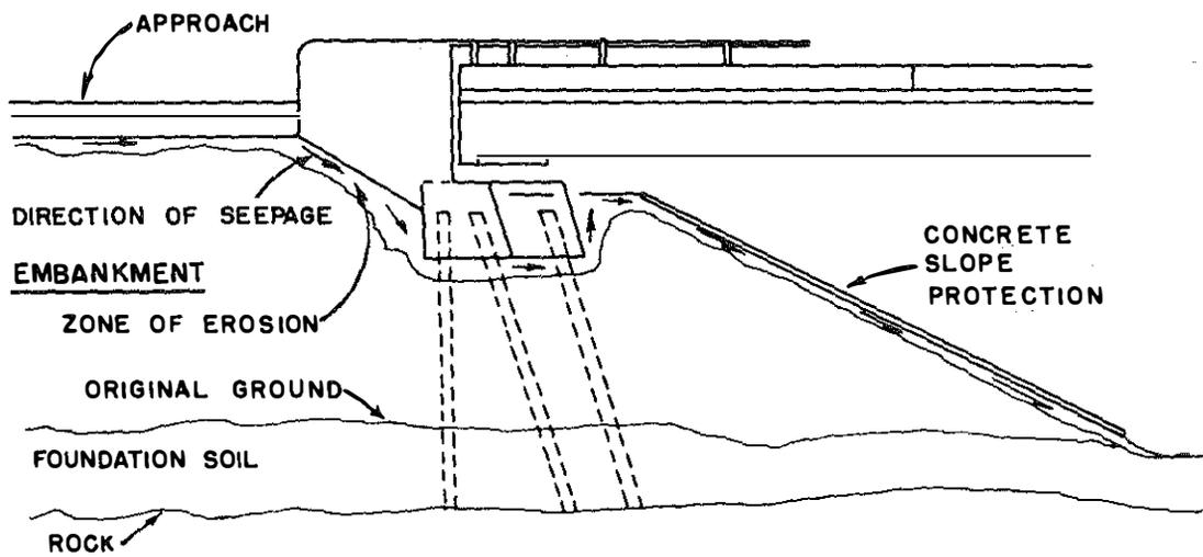
Figure 10 Direction of Seepage and Zone of Erosion
