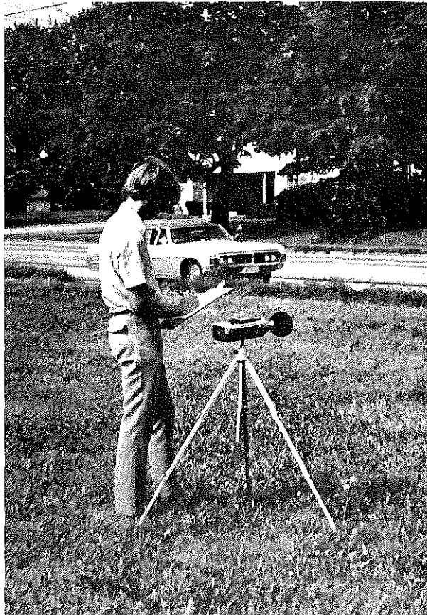
Figure 2. Typical Field Monitoring Arrangement Used in Data Collection.
