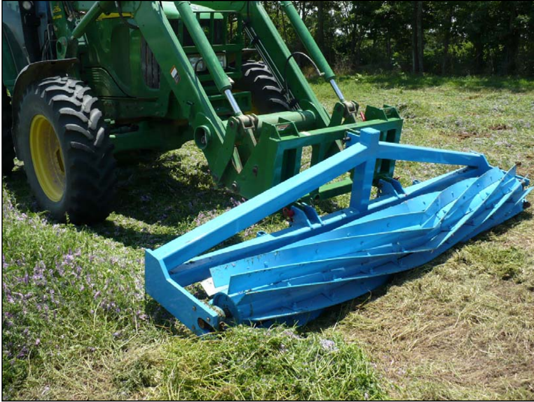
Figure 1.1. Roller crimper constructed by the University of Kentucky based on Rodale Institute plans.
