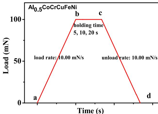
Figure 1. Schematic of indentation load vs. time.
