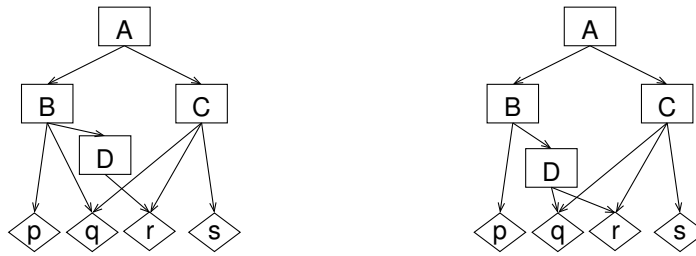
Figure 3.18: Inserting a node into a GODDAG. Both documents result from inserting q into Figure 3.17 as a child of C preceding r ; only the document on the right is a range GODDAG.
