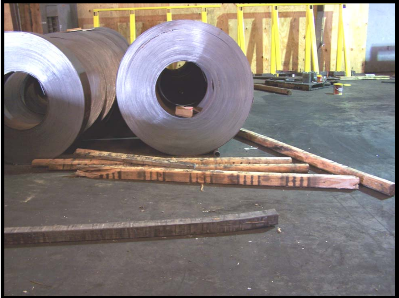
Photograph showing coils of slitted steel with boards to be used as chocks.
