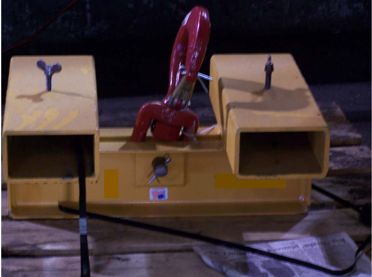
Picture of device workers should have been using with the forklift to transport coils of steel.
